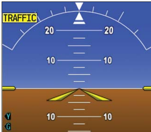
Figure 5-35 Pitch Scale with SVT Disabled
